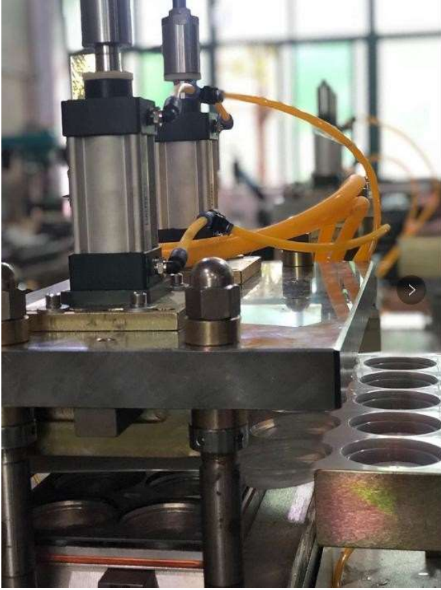
Forming Part Hole or Cross Punching Part
