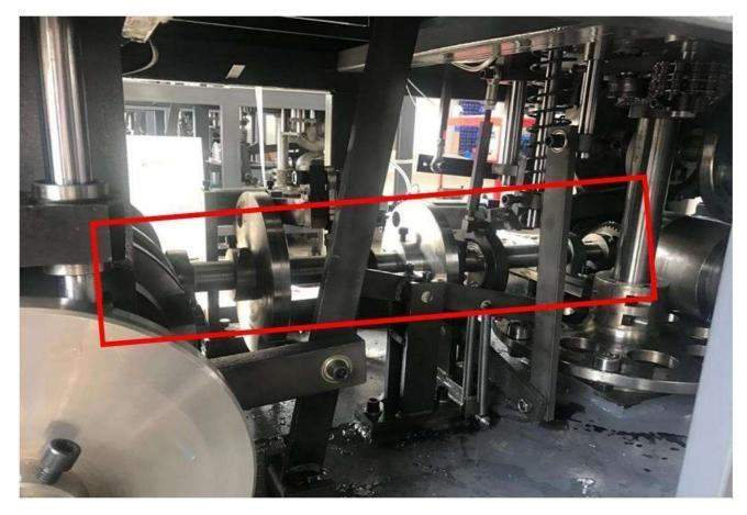
Automatic Oil Lubrication System for oil lubrication machine moving spare parts which to make sure machine running high speedbut spare still keep long span life
