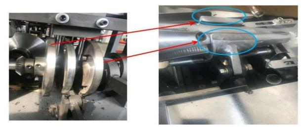
The Left Cam is for controlling the left closure holder. The Right Cam is for controlling the right shut-off holder.
