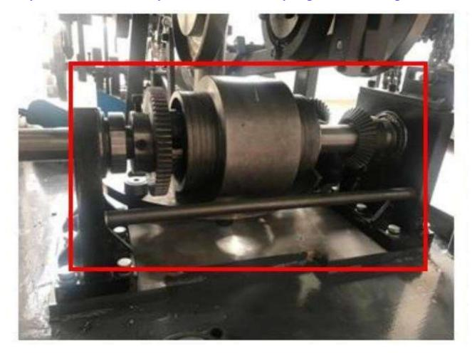
The main mechanism and moving parts are controlled by quality gears, which are more efficient and stronger than the chain and axis.
