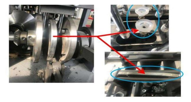
The middle Cam is for controlling Sucker and Rod Hold paper fan End-to-end Single Shaft in-machine to control the whole machine not difficult to operate and broken and easy to check When the machine is running
