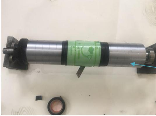
Flexo Plate can be glued on printing cylinder by this machine
