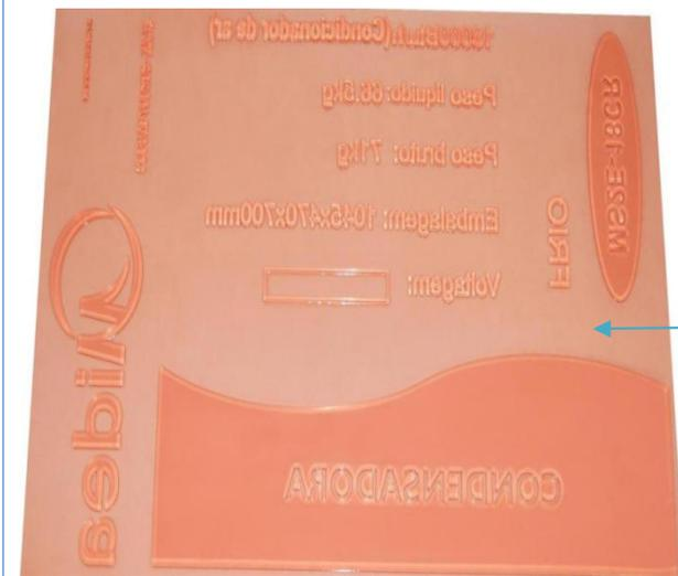
**Printing cylinder stucked with Flexo plate**
