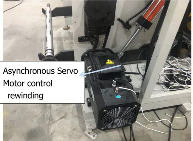
Asynchronous Servo Motor control rewinding
