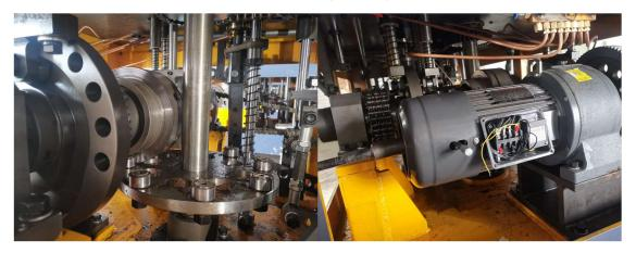
B. Machine has full automatic lubrication by oil pump and filtration, more convenient formaintenance.
