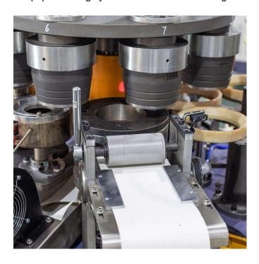
G. New-type stable collecting system solves the collecting problem of the paper bowl totally, reduce the packing labor and improve the working efficiency,
