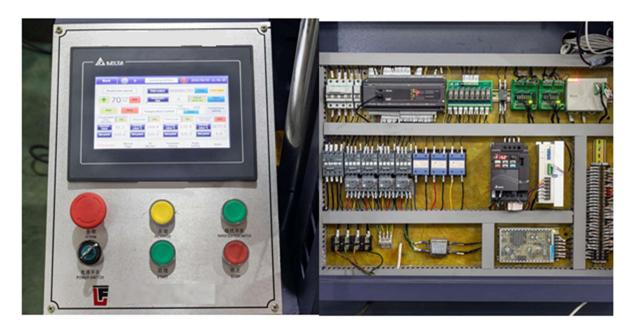
E. The machine is controlled by PLC, and has a encoder to control the working of ultrasonic, sensors, solenoid valve and so on, to make the running of each process more accurately.
